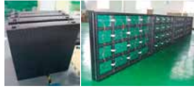
Complex structure, More cables, Unable to be modular.
